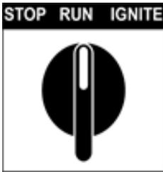
**Starting** and **stopping** the burner can also be done with the optional **manual Start/Stop** switch. There are **three** functional positions as shown. When in the stop position, all safety outputs are de-energized. Toggling from the **Run** position to the **Ignite** position for more than **2 seconds** initiates the ignition sequence. Toggling the switch from the **Stop** position to the **Run** and back to the **Stop** position can clear a lockout state.
